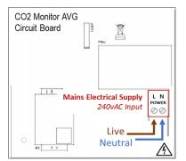
A 240VAC Live and Neutral electrical supply should be connected to the terminal marked [POWER] as shown.
